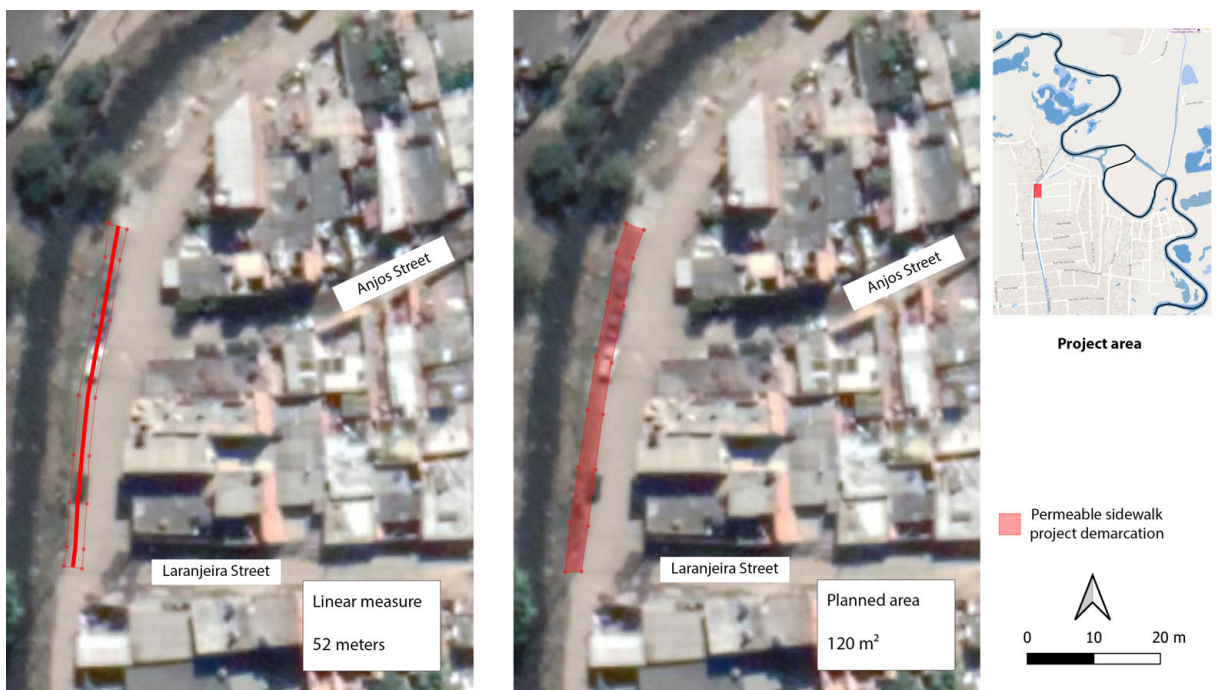
Fig. 22: Dimensions of the areas available for the proposed sidewalk to Cachoeira de Itaguassava Street. Source: Authors, 2021.
