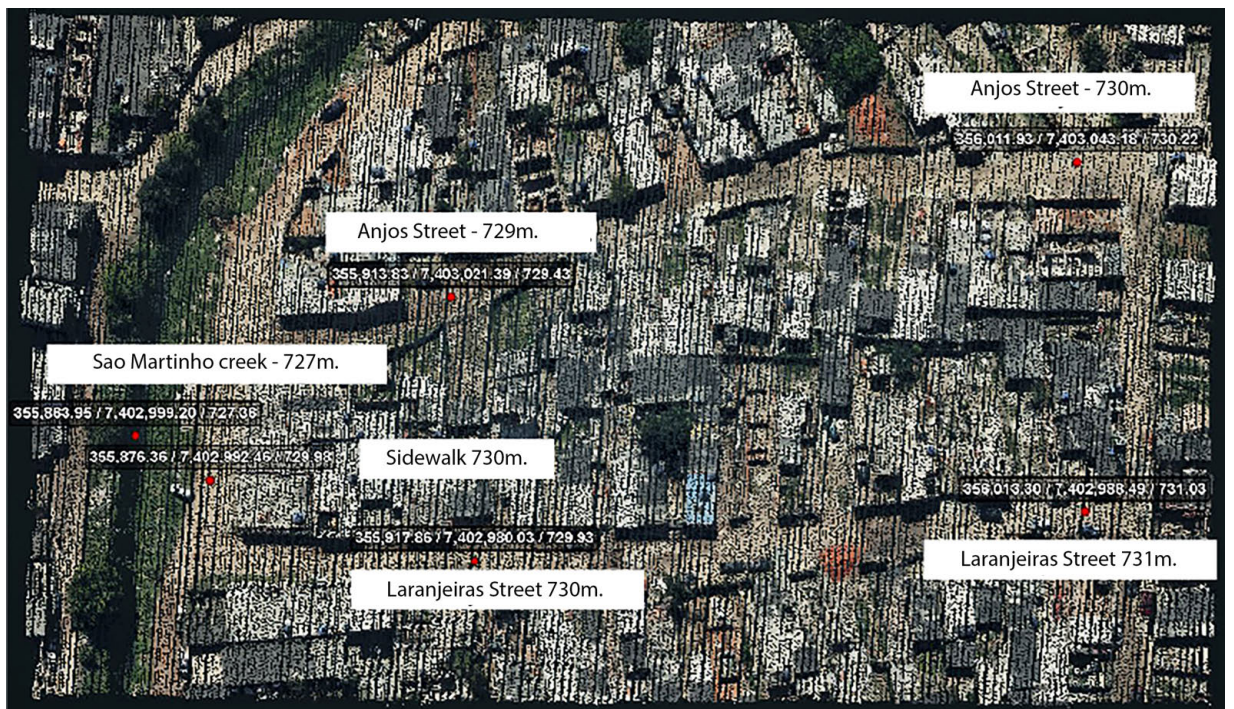
Fig. 21: Altimetry of the streets that flow into the São Martinho creek. LIDAR — Estudio Laborg. Source: ZL Vortice Project, 2020. Available at: https://zlvortice.wordpress.com/ . Accessed: 25 February 2021.
