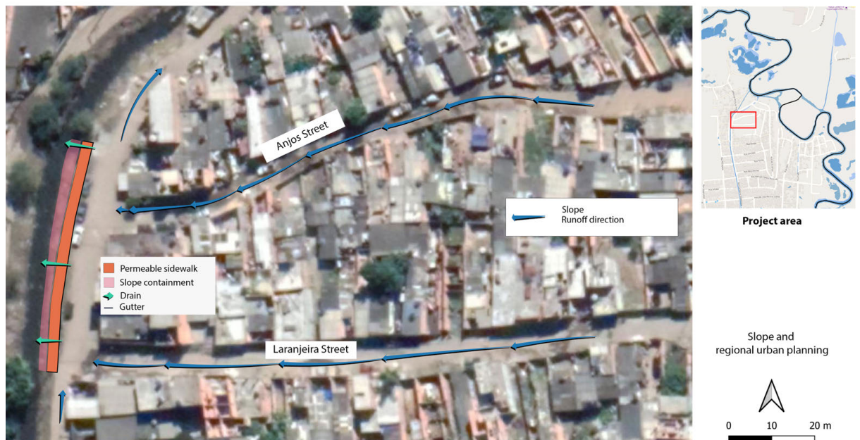
Fig. 23: Schematic map of the surface runoff in transversal streets converging on the sidewalk and urban design of the area, with contention of the stream margin, gutter, manholes and drain. Source: Authors, 2021.
