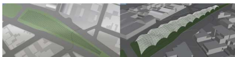
Fig. 8: Code 1 programmed on Grasshopper: It defines the main pavilion’s roof and structure. Source: Research archives, 2018.
