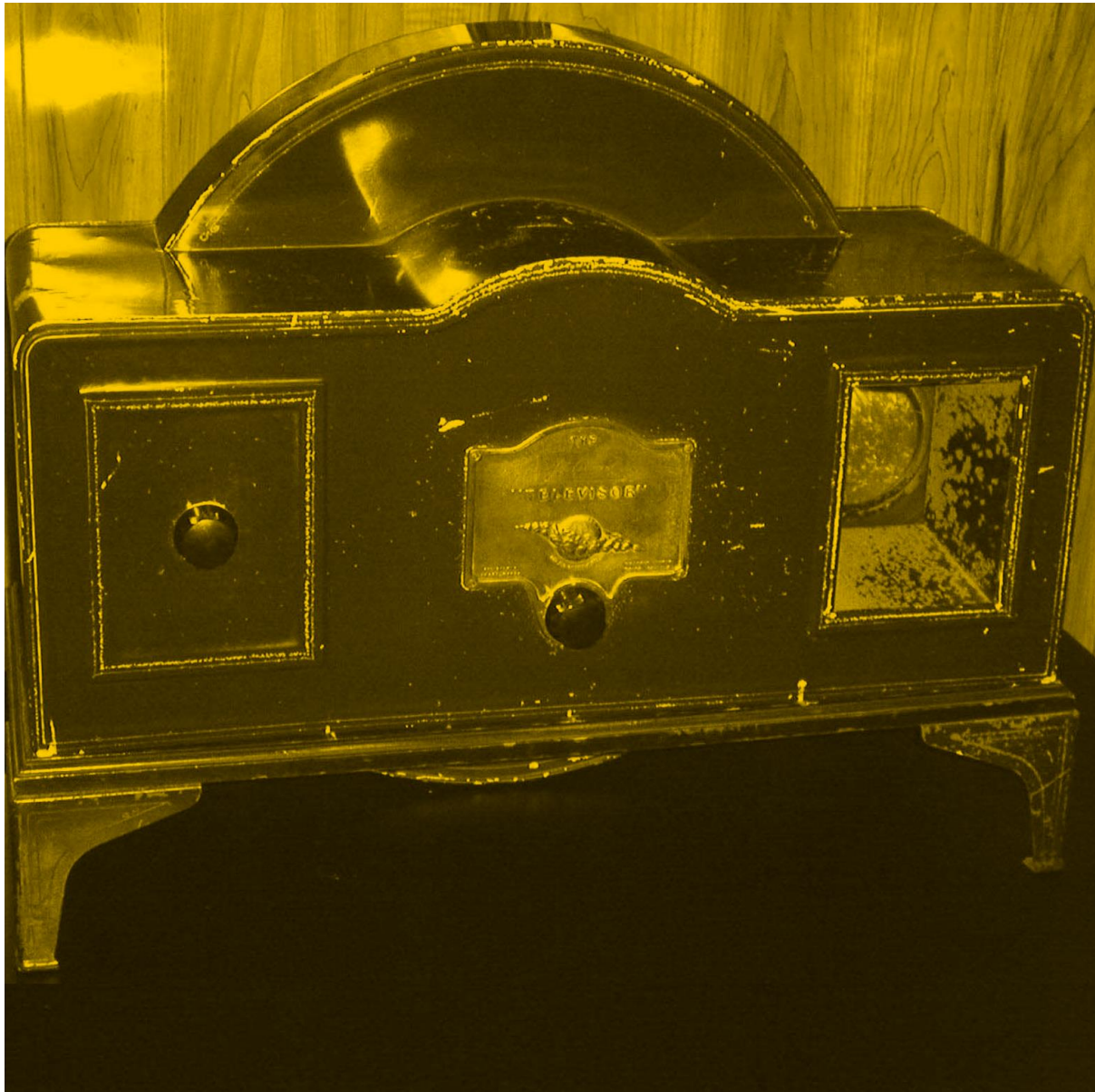
Fig. 07: The televisor invented by John Logie Baird in London in 1926.
