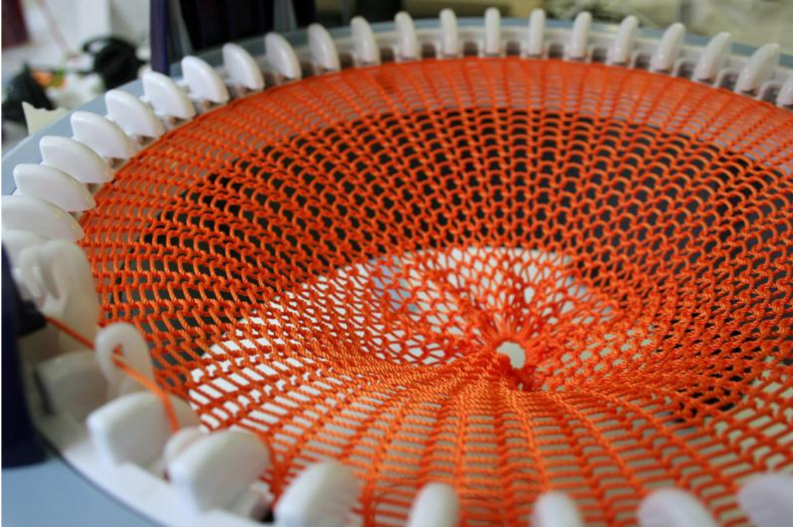
Figure 1. Household Circular Knitting Machine.
