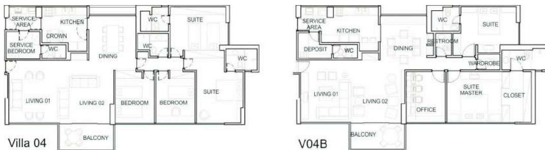
Figure 15. Example of an assemblage of two bedrooms to form a master suite and to introduce a home office.
