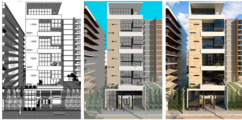
Fig. 1: Simulation of different stages of pictures produced by three-dimensional digital models. Modeling made in SketchUp 2017 and rendered in V-Ray 3.4. Source: By authors, 2019.
