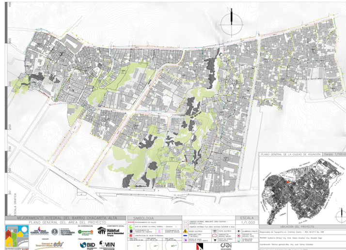
Fig. 9: One of the final products. High precision CAD plane, with deviations of +/- 15cm. Source: CIDI.
