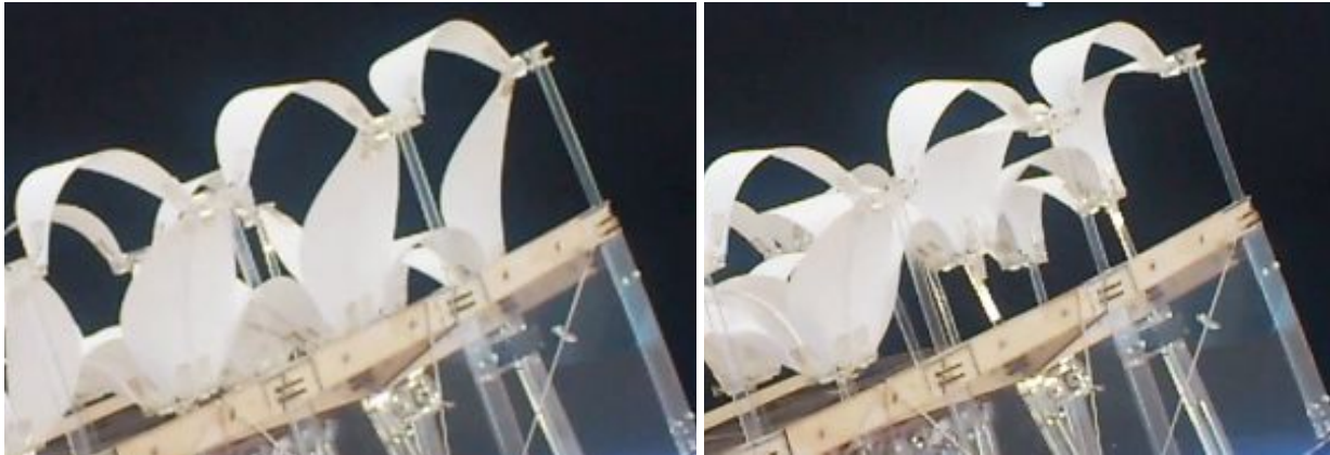
Figure 2: Hyperbody MSc 4 project featuring interactive building skin components employed for ventilation purposes.
