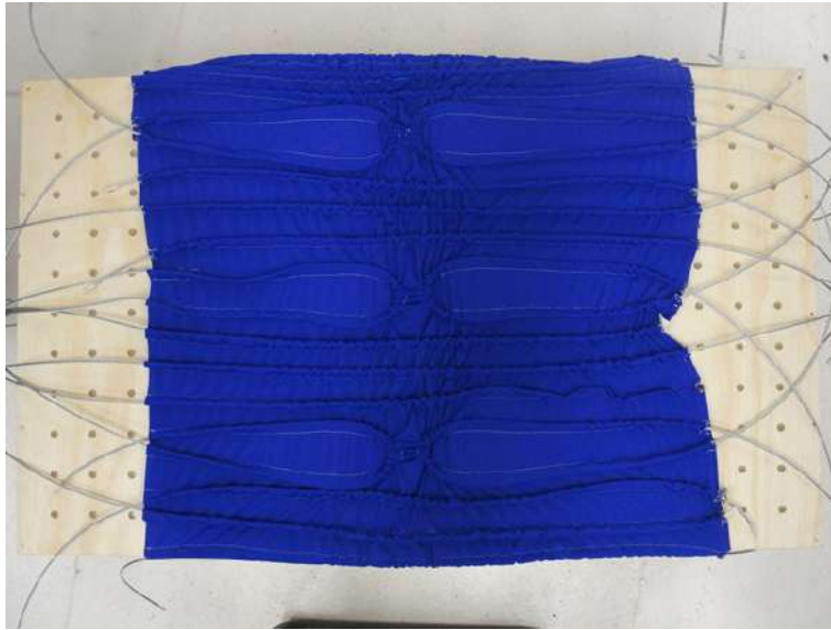
Figure 8. Sewing standard for the passage of cables in elastane.
