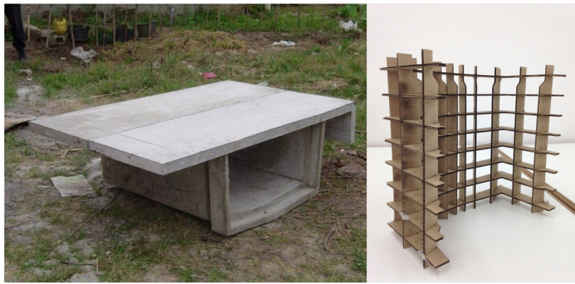
Fig. 3: Module and mold digitally fabricated. Source: Projeto ZL Vórtice, 2017. Available at: https://zlvortice.wordpress.com/ . Accessed on 05/06/2020
