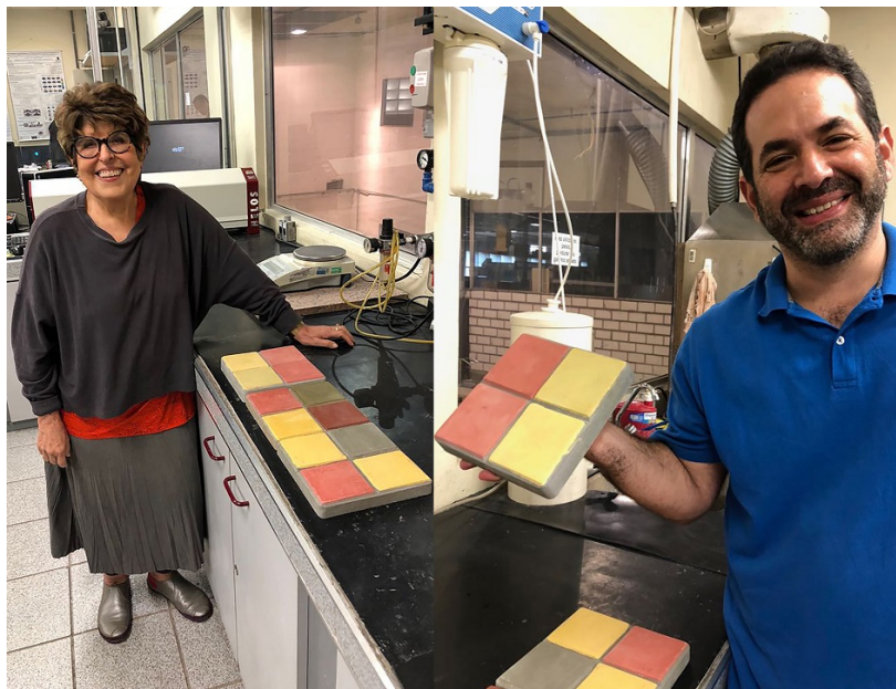
Fig. 11: Manufacture of a test model on a reduced scale of the interlocking pavement. Source: Projeto ZL Vórtice, 2018. Available at: https://zlvortice.wordpress.com/ . Accessed on 05/06/2020
