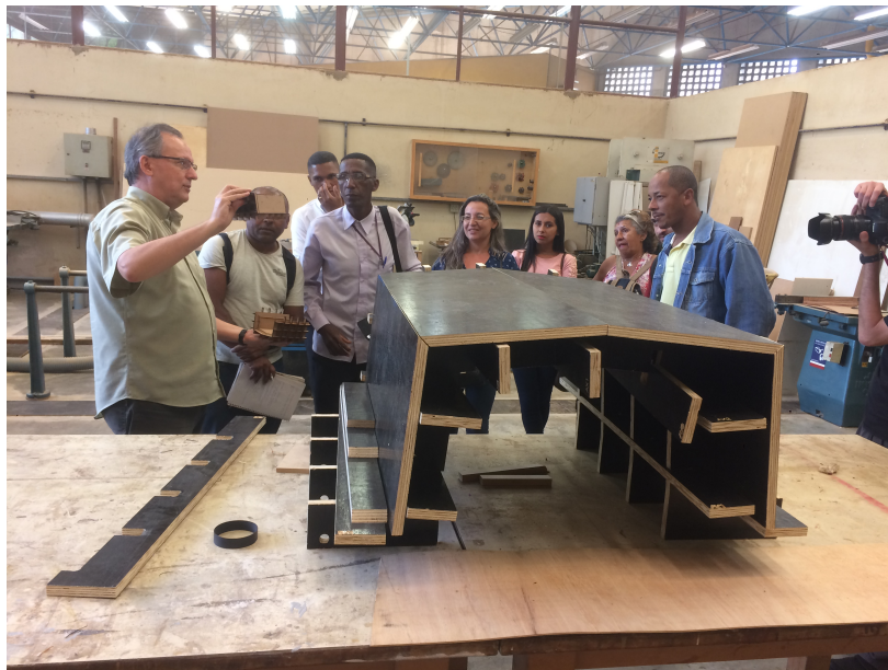
Fig. 4: 1:1 scale prototype of the drainage gallery module. Source: Projeto ZL Vórtice, 2018. Available at: https://zlvortice.wordpress.com/ . Accessed on 05/06/2020
