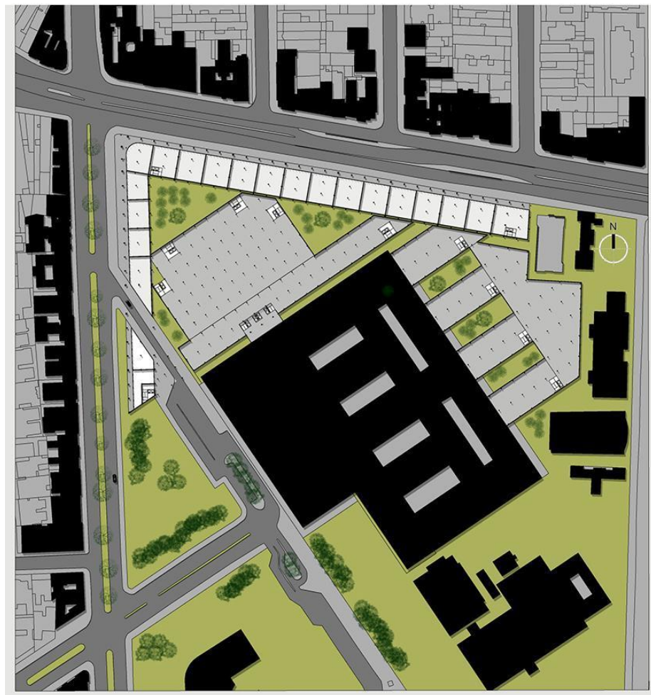
Fig. 15: HCPA, counter-project. Ground floor plan, commercial areas in white. Source: The author, 2020.
